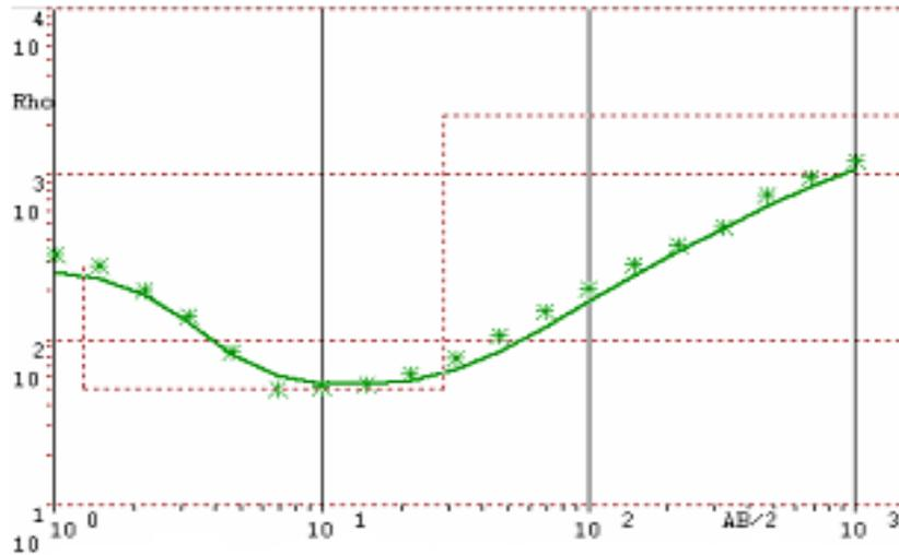
**Figure 04:** Interpreted model of Observed and computed resistivity Schlumberger depth sounding data from the VES 130 forward modeling program, at the 600m mark point along profile 1.
