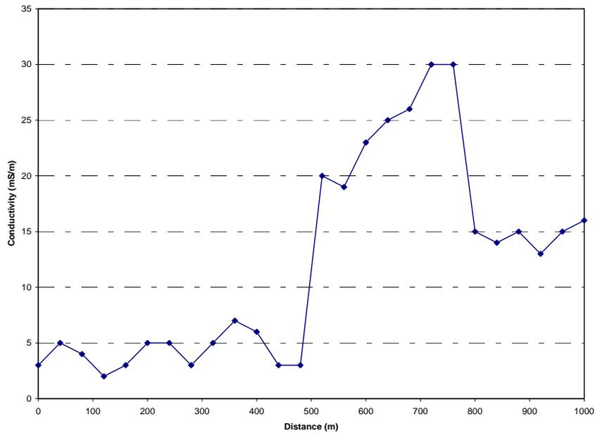
**Figure 01:** Plot of EM34-3 data from profile line 01 in the study area.
