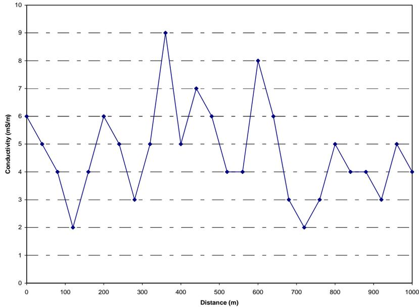
**Figure 03:** Plot of EM34-3 data from three profile line 03 in the study area.
