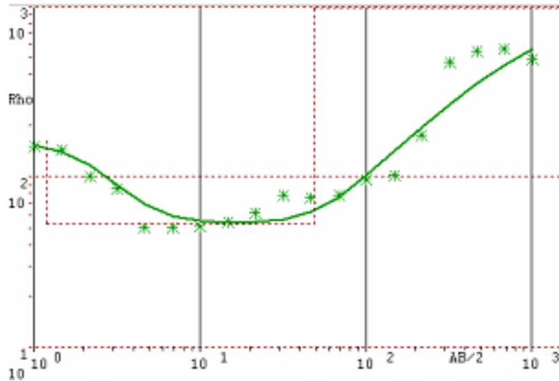
**Figure 05:** Interpreted model of Observed and computed resistivity Schlumberger depth sounding data from the VES 130 forward modeling program, at the 750m mark point along profile 2.
