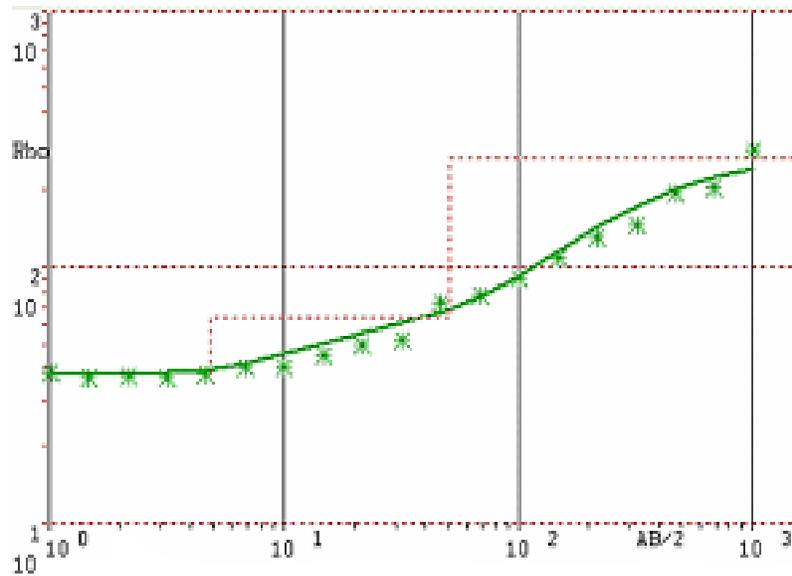
**Figure 06:** Interpreted model of Observed and computed resistivity Schlumberger depth sounding data from the VES 130 forward modeling program, at the 500m mark point along profile 3.
